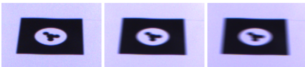
(a) Exposure time is 15 ms (b) Exposure time is 30 ms (c) Exposure time is 45 ms
