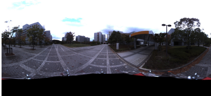
Fig. 1. Omnidirectional panorama image with missing region (black region) caused by the blind side.
