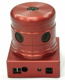
Figure 3.8. Omnidirectional multi-camera system "Ladybug".
