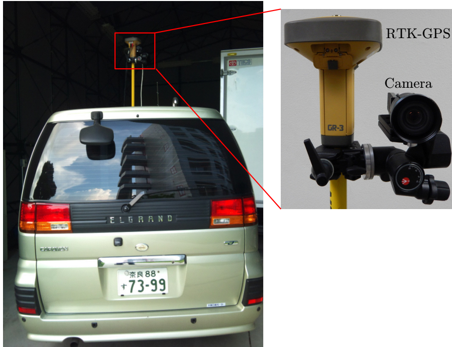
Figure 2.5: Camera and RTK-GPS mounted on the roof of a vehicle.
