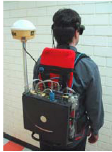
(b) Backpack including GPS and IMU [60]
