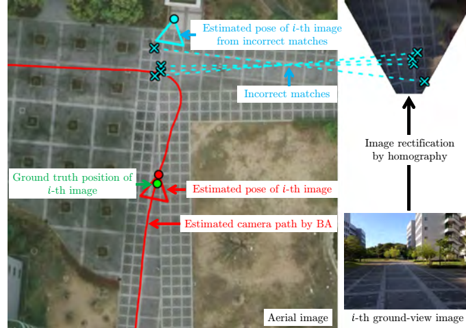
(b) Global geometric verification. Blue dashed lines are incorrect matches obtained by RANSAC with a scale and orientation check. The red line and triangle represent the camera path and pose estimated by BA using sampled matches, respectively.
