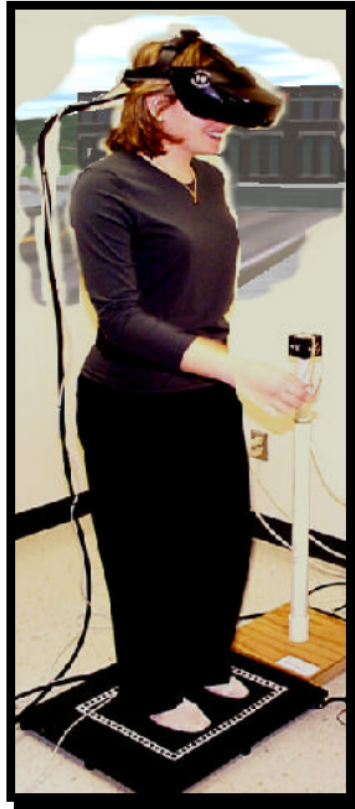
図 11 The Pressure Mat[31]
