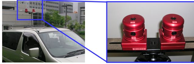
Fig. 2. Omni-directional multi-camera systems mounted on a vehicle
